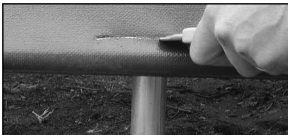
Making Slit and Installing Side Ratchet Strap
