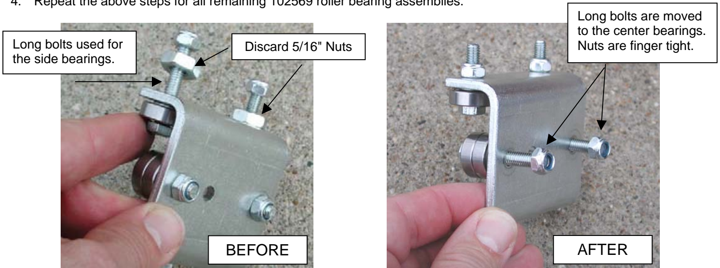
Before: Long bolts on side bearings.
