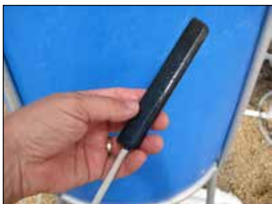
Slide 111046A tube onto air stone. Wet hose or nipple on stone for easier installation.
