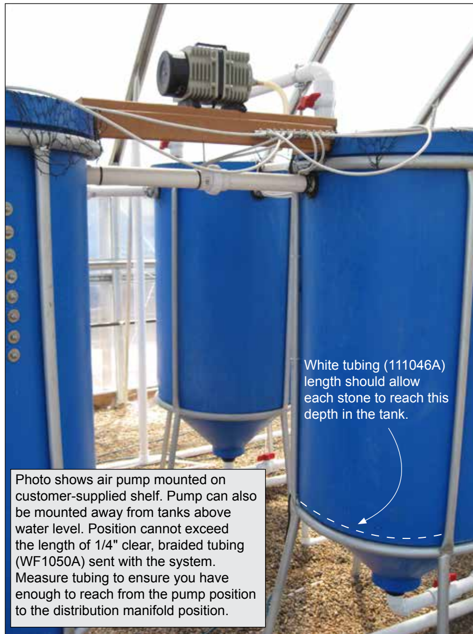
Photo shows air pump mounted above water level. Example only.
