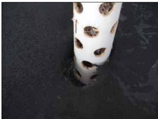
1. Slide siphon tube down into tank and over the standpipe.
