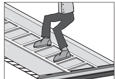
Warning! Do not step on the sheets between the purlins! Figure 23
