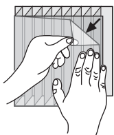
Figure 17a. Partial or Complete Removal of Protective Film Prior and after Installation
